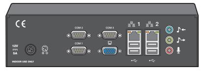
The AIM server rear panel. In normal use only the network and power connectors are used.
